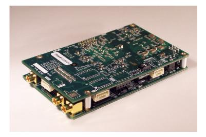
The Discovery 60 PCB uses an FPGA in addition to dual-core processor technology to provide a powerful FPGA+DSP platform capable of executing a complete suite of real-time video image- processing functions simultaneously. It also includes an ARM-9 general-purpose microprocessor running embedded Linux for robust user-interface and control implementations.
