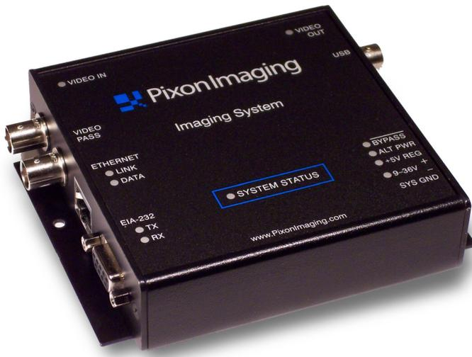
The Discovery 40 employs multi-core processor technology to provide a powerful DSP platform capable of a wide range of real-time video image-processing functions, along with an ARM9 general-purpose microprocessor running embedded Linux for robust user-interface, control, and peripheral implementations.
